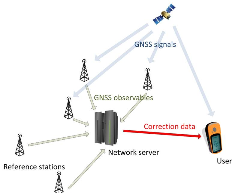
Figure 1. Structure of a ground-based augmentation network
