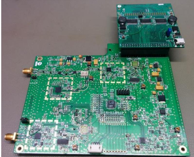
**Figure 1.6 Adapter board with custom USB interface for long captures**
