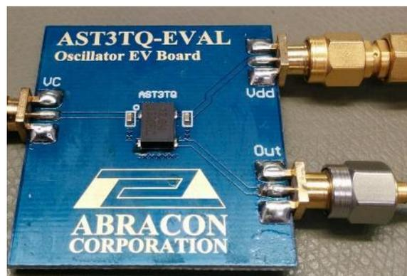
**Figure 1.25 Additional board utilized for external TCXO**
