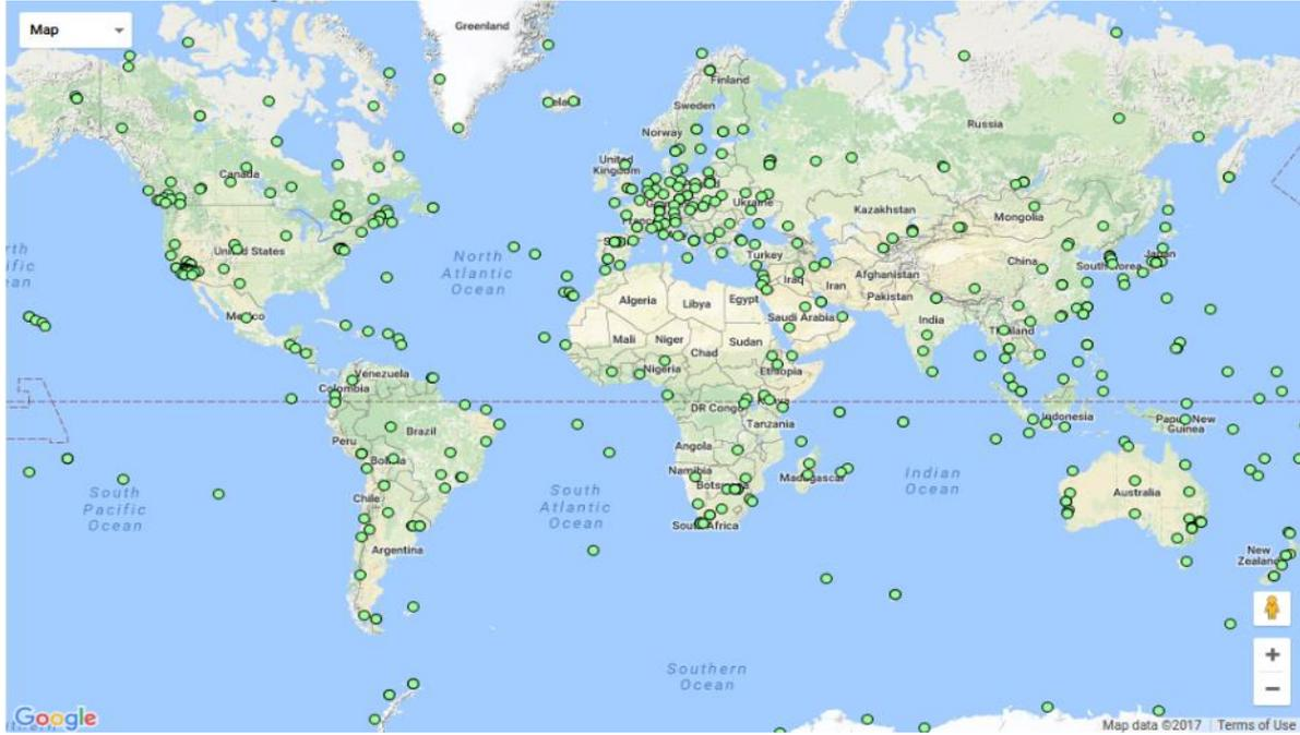
Figure 3.4: IGS network with globally distributed stations with high coverage over Europe and huge data gaps over the oceans. However, meanwhile several islands are worldwide equipped with GNSS receiver stations.
