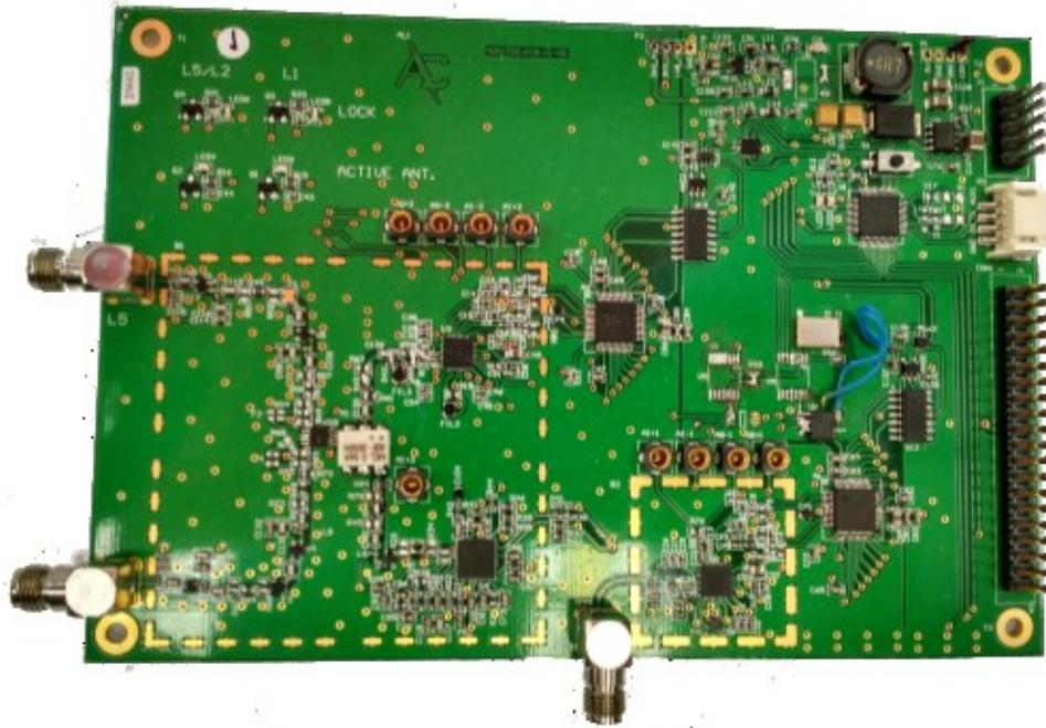
**Figure 2.5: FE v1.0 PCB top layer**
