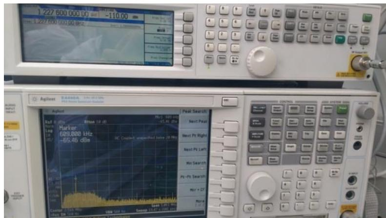
Figure 2.9: FE v1.0 measurement, GPS L2 band single tone, IF at 609 kHz (BW 2.5 MHz).
