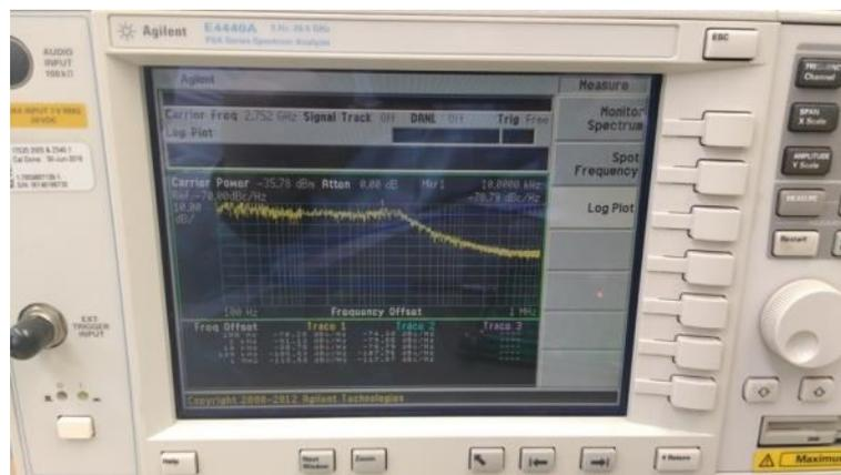
Figure 2.11: OL phase noise measurement.
