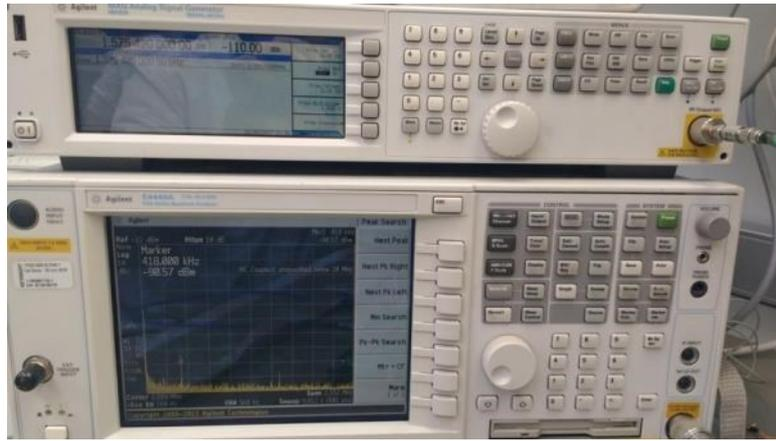
Figure 2.8: FE v1.0 measurement, GPS L1 band single tone, IF at 418 kHz (BW 2.5 MHz).
