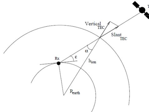
**Figure 3.1: Thin layer model scheme where the relation between the STEC and VTEC can be seen graphically.  $R_x$  denotes the receiver while  $T_x$  denotes the transmitter.**
