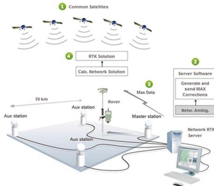
Figure 3.13: MAX network architecture given a rover receiver (from [http://uk.smartnet-eu.com/max-corrections\\_233.htm](http://uk.smartnet-eu.com/max-corrections_233.htm) [68])
