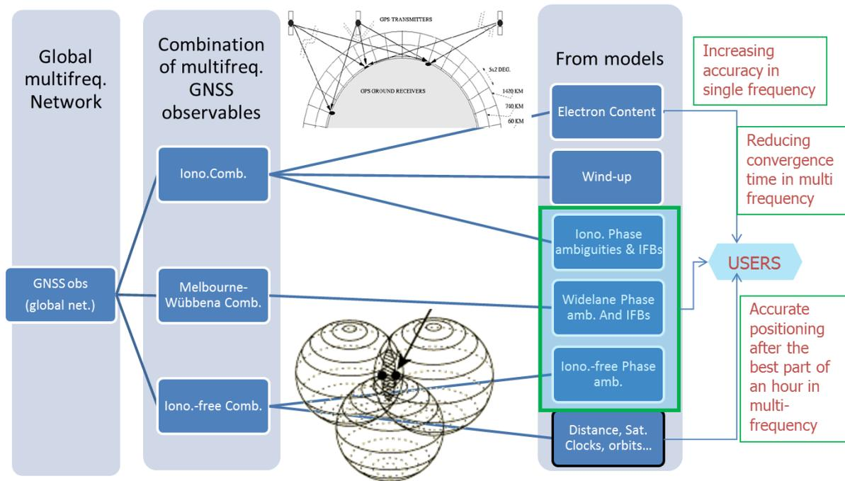
**Figure 3.8: Diagram showing the main processing steps of WARTK and FPPP approaches, including phase ambiguity resolution.**
