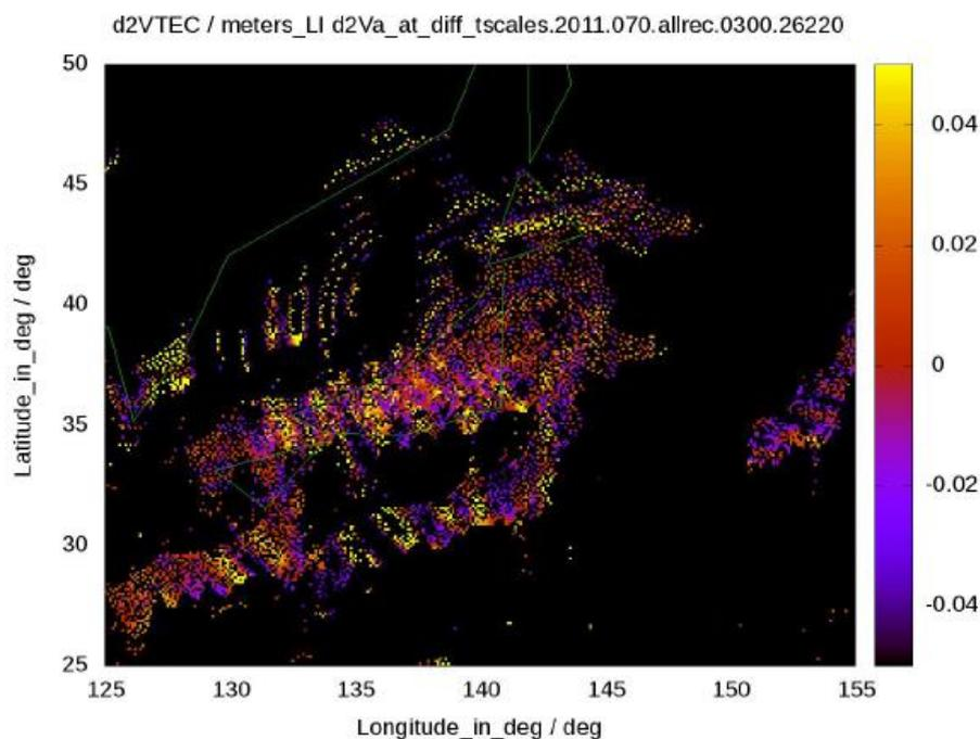
**Figure 3.5:** Detrended VTEC obtained from GEONET GPS data, coinciding with the Tohoku earthquake and tsunami (GPS second 26220 of day 70, 2011), where the circular ionospheric waves centered at the earthquake epicenter are evident (extracted from Hernández-Pajares 2013 [98]).
