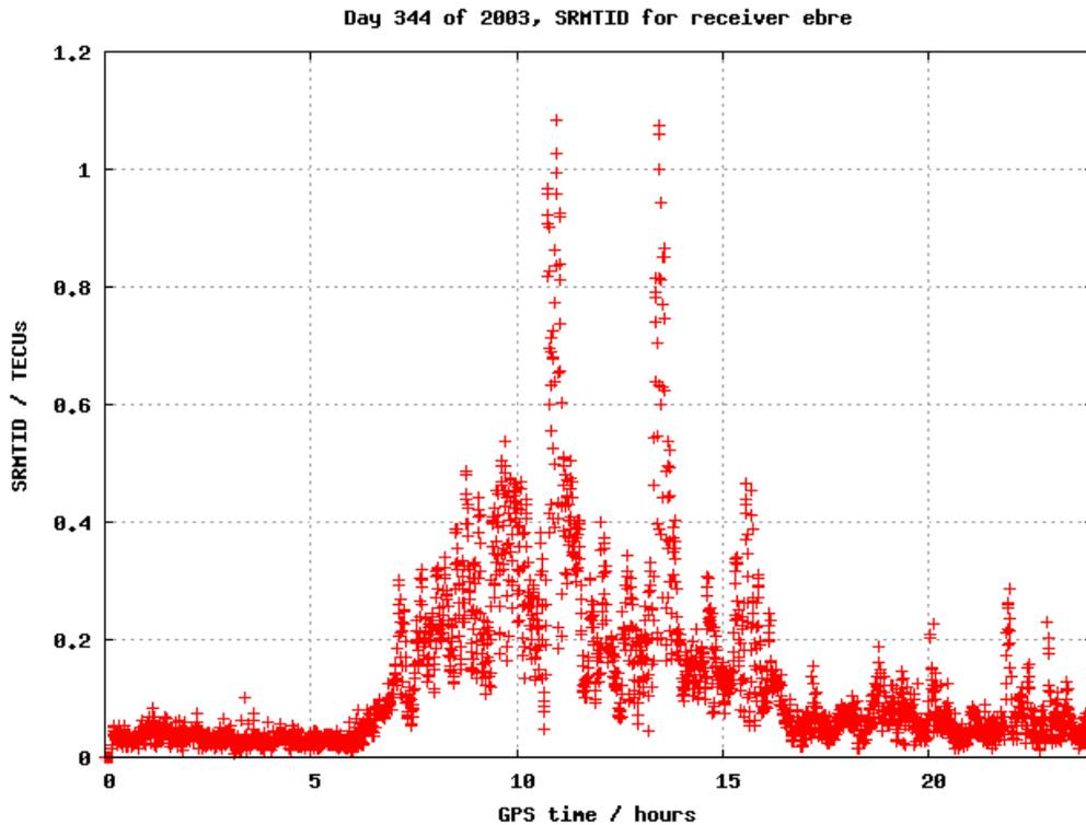
**Figure 3.6: Example of SRMTID index corresponding to receiver EBRE during day of year 344 in 2003.**
