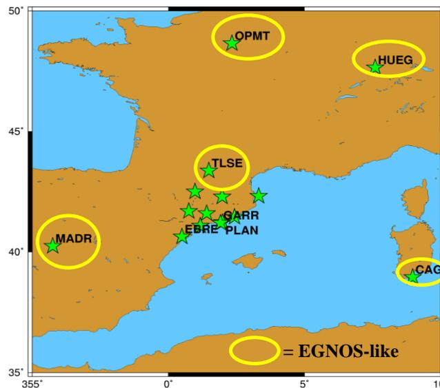
**Figure 3.10: Map indicating the reference receivers: highlighted in yellow for the case of a large network, and the remaining labelled ones for the case of a small network; the remaining receivers (not labelled) are treated as roving users.**
