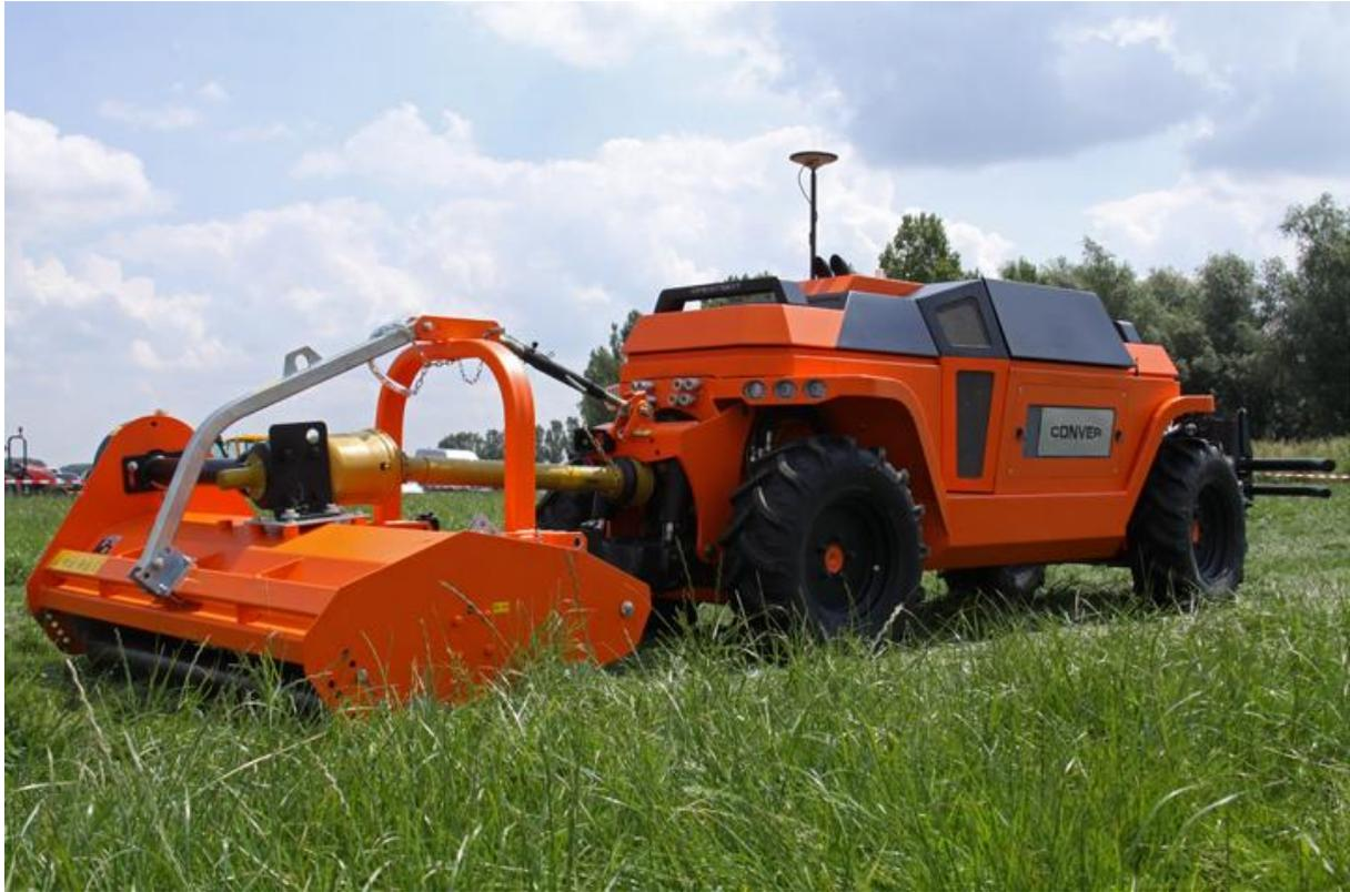
**Figure 4.6: Conver Greenbot – autonomous mowing robot ([35])**
