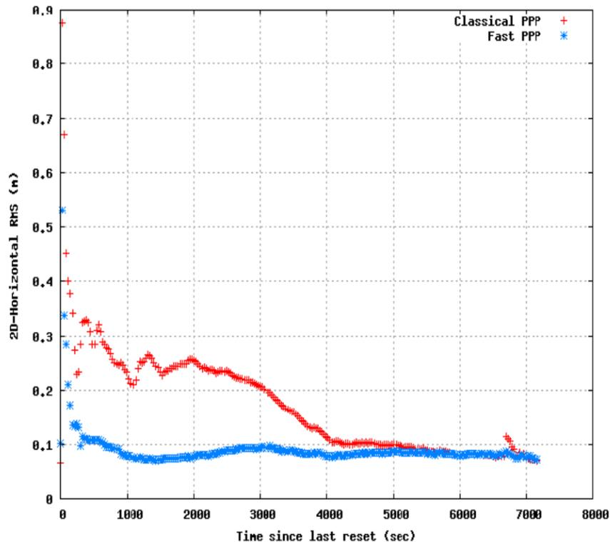
**Figure 3.11: Comparison of classical PPP (red) and Fast PPP (blue) convergence of positioning error.**
