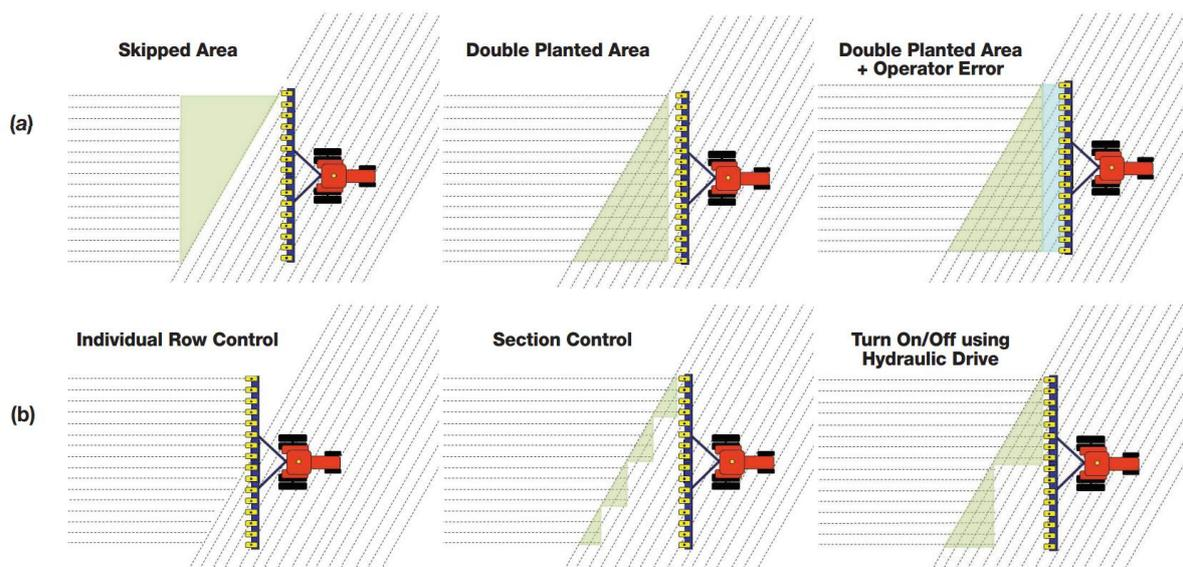
**Figure 4.4: A comparison between using a traditional machine setup where the operator must decide to stop planting (a) versus one equipped with automatic section or row control (b) reducing overlap and skipped areas ([33]).**
