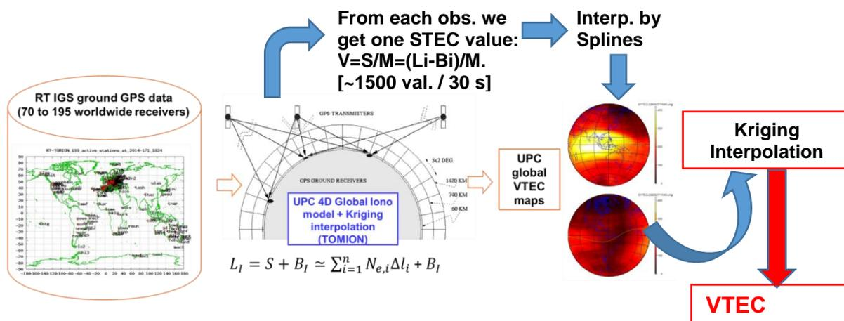
**Figure 3.3: Layout summarizing the global VTEC computation from ground GPS data by means of the UPC TOMION software, including the main tomographic model equation (data: ionospheric combination of carrier phases (Li) and length intersection within each voxel (Δli); unknowns: its ambiguity (Bi), the STEC (S), which includes the mean electron density within each given voxel (Ne,i).**
