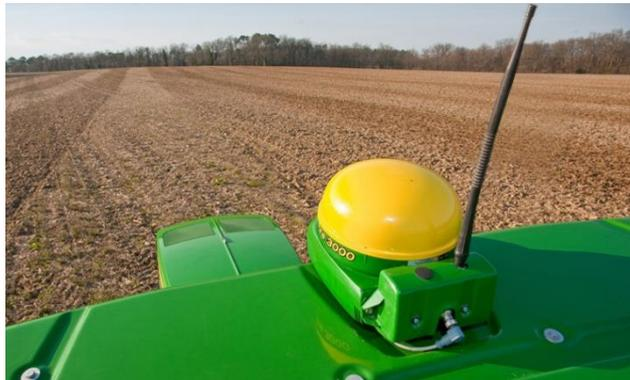
Figure 3.17: StarFire receiver on top of a tractor (from <http://www.deere.com> [70])
