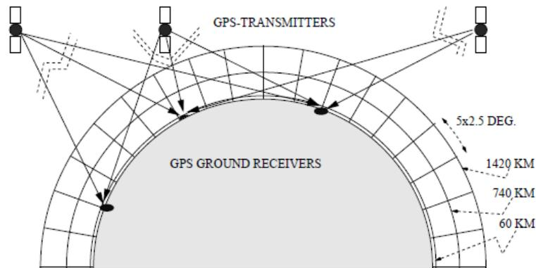
**Figure 3.2: Two-layer voxel model used in the computation of TEC at the UPC. From Orús 2005 [116].**
