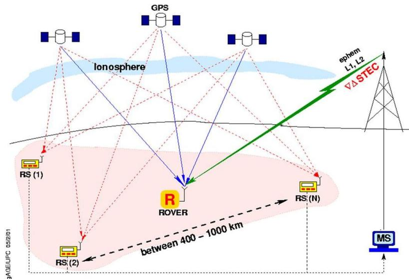
**Figure 3.7: Layout representing the main components of the WARTK system: The Central Processing Facility (CPF), continuously running the combined geodetic and ionospheric models, both feed with the measurements of the permanent stations.**
