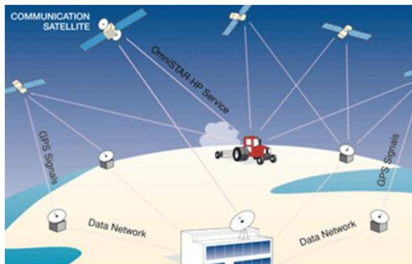
**Figure 3.16: Omnistar architecture providing support to precise agriculture**
